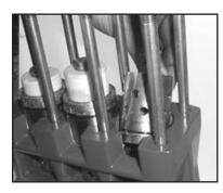
10. For LP122A & LP122A-4000 pumps, generously lubricate the inside of the oil seals (31A & 33) and o-ring (32A). Next, place the seal retainer, complete (31) over the steel plunger base seat firmly into the crankcase. Replace the flinger (30).
